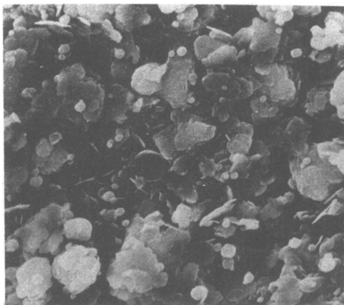
Fig. 6 SEM of C_3A paste hydrated 2 hours without addition, magn. 5400 ×
